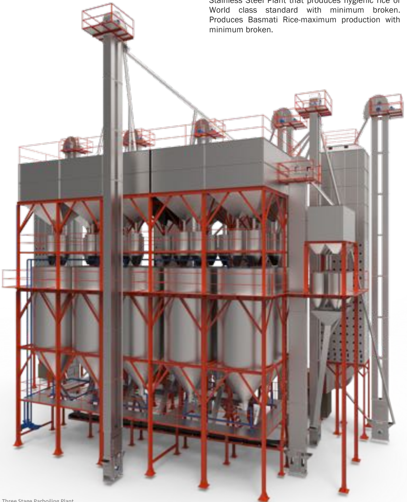
Three Stage Parboiling Plant with Post Steaming (Pakki) on the side.
