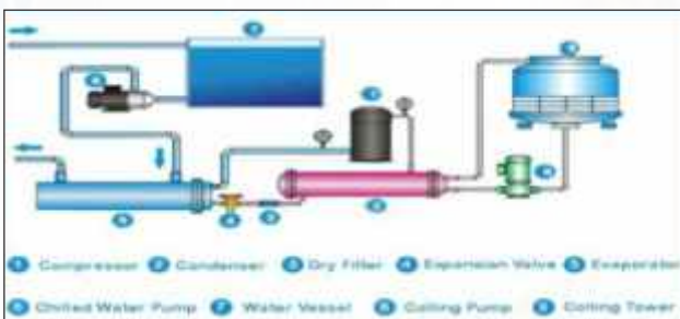
Water Cooled Water Chiller
