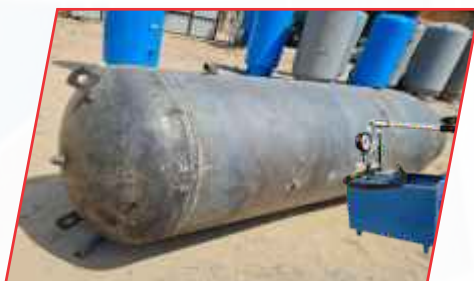
Hydro Testing upto 70 Kg/cm 2 Pressure
