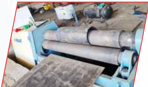
PLC Controlled Hydraulic Rolling Machine (Rolling upto 18mm thickness)
